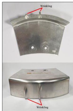
Figure. 5: A formed specimen sample with wrinkling defect (material: AA2024-W, thickness: 1.27mm, contour radius: 125mm, flange length: 40mm).
