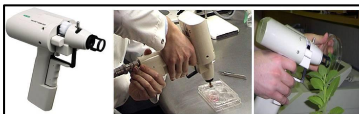
Figure. 2: Gene gun Helios TM by BioRad is used to transfect cells in cultures and plant leaves
