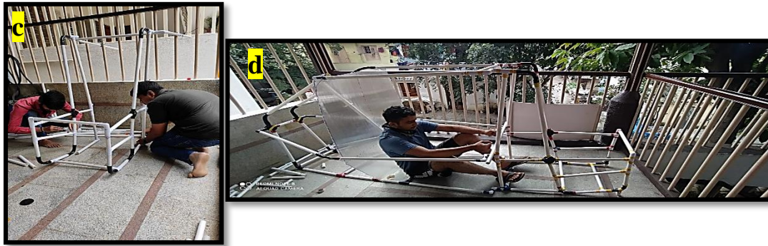
Figure. 1: a b c Shows the Initial Fabrication of ATV and D the Final One by Using PVC Pipes
