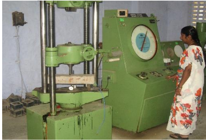
Figure. 4: Set up of flexural strength test
