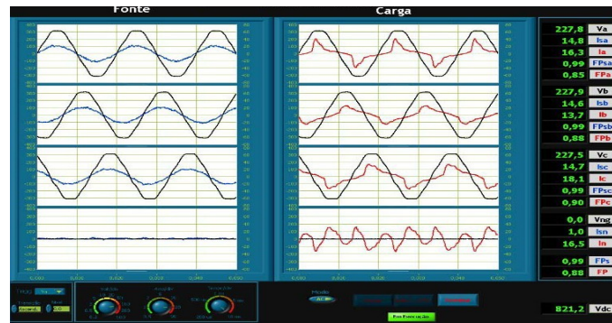
Figure. 3: System voltages and currents waveforms at Load and Source sides, registered in installation 2 (Computational Centre)
