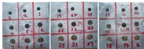
Figure. 6: Drilled Specimen with Markings Machine (2.5%, 5%, 7.5%, from left to right)
